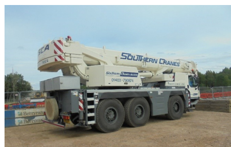
An example of the type of crane that will be required for the installation of sheet piling
